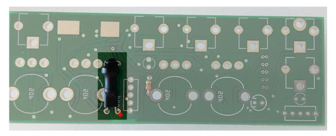
Note the red dot, that's where the short leg should go. Since there should be room for a pot just to the left of it, you should make some slack or even place the pot (no soldering) to make sure you have the room for it later.
