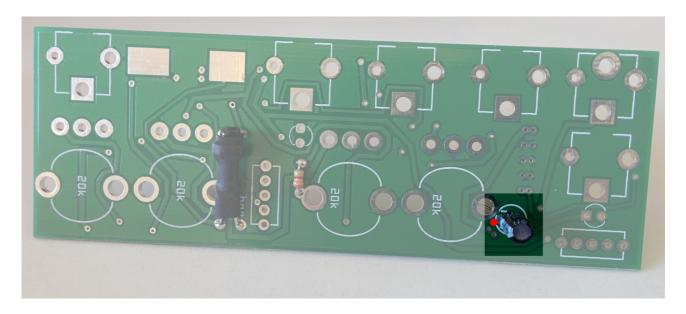
The other cap goes on the other side of the PCB and has to be soldered on the SMD pads close to the large pre-soldered IC. Short leg goes (negative lead, marked on the cap with a white stripe) on the pad with the red dot, long leg on the pad with the yellow dot.
