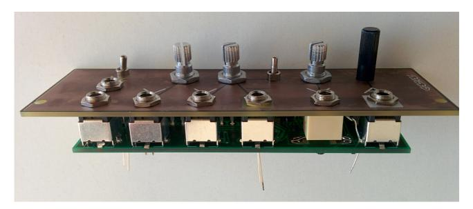
Turn the board over and solder all jacks, pots and the two LEDs. You might want to pull the LEDs just a tad away from the panel before soldering, leaving about 1mm of space between the LEDs and the panel. Cut off the excess resister leg and the LEDs legs.
