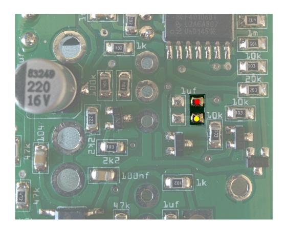
Cut the legs of the cap short. Obviously, from now on, you won't know which leg is the short leg, except from looking at the white stripe, which is where the short leg used to be
