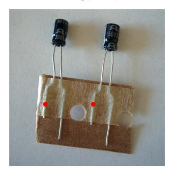
The short leg (also marked on the cap with a white stripe) is the negative lead, and should go into the hole marked – on the PCB. The two caps go on each side of the PCB. First place and solder the one on the same side as the resistor and the vactrol, note the red dot, marking the short leg:
