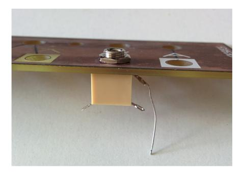
Turn the panel over and apply a blob of solder on the two legs (not the one with the recycled reresistor led soldered to it)
