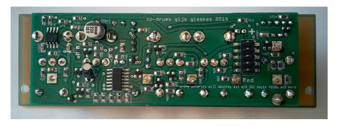
Now solder the lonely jack to the pads, by pressing the jack legs against the pads with the hot iron.
